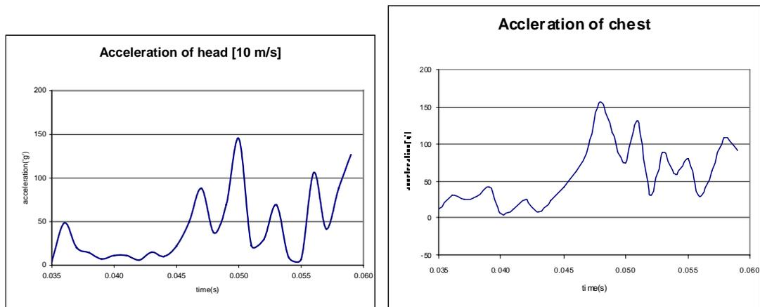
Fig. 4. Acceleration during impact: (a) driver head ; (b) driver chest
