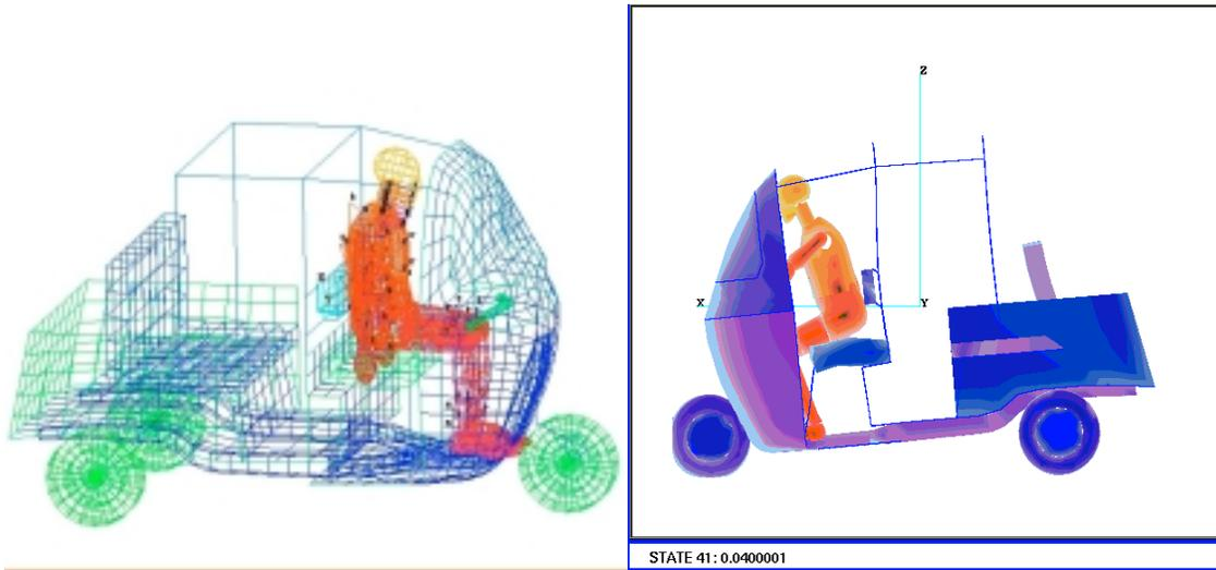
Figure 1: FE model of the TST with the driver: (a) position before impact; (b) positions 40msecs after impact with front rigid wall
