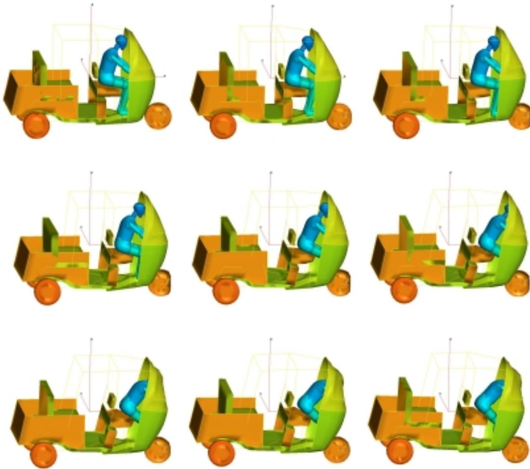
Figure 3: The kinematics of the TST – wall crash with the driver.
